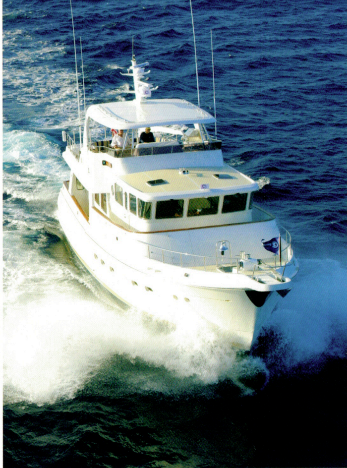
Barely visible below the surface in this picture taken off the bow, Southern Pearl has the optional bulbous bow, which combined with KeyPower fin stabilizers, improves ride in heavy seas. Above right, generous cockpit seating will keep the captain in the heart of the gathering. Below right, the gentle sweep of the stern can be seen in the curved bench seat with cockpit table.
