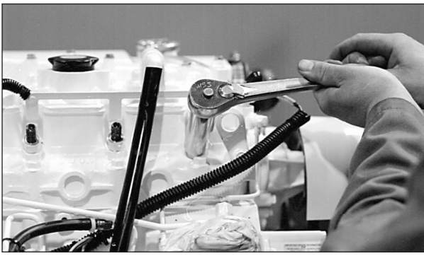
Figure 18: Reinstall injector. Torque to proper tightness.
