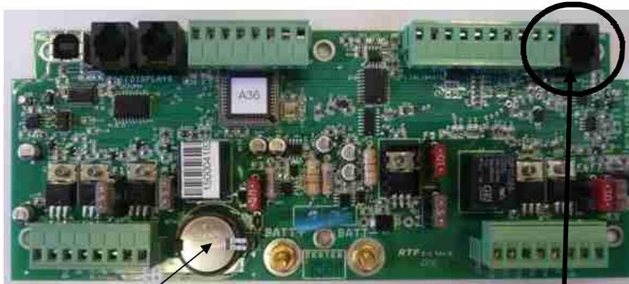
Remove the battery isolation tab after installing the salinity probe
