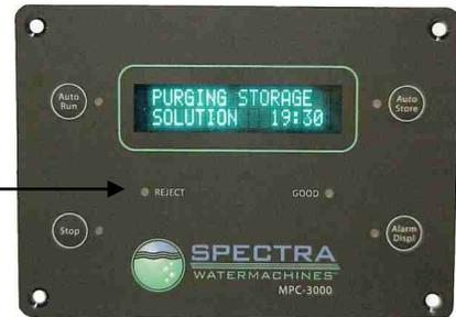
**Note:** You can bypass the purge sequence and initiate a normal start at any time by Pressing “Auto Run” and “Stop” simultaneously. This will bypass the purge sequence and enable a normal start.
